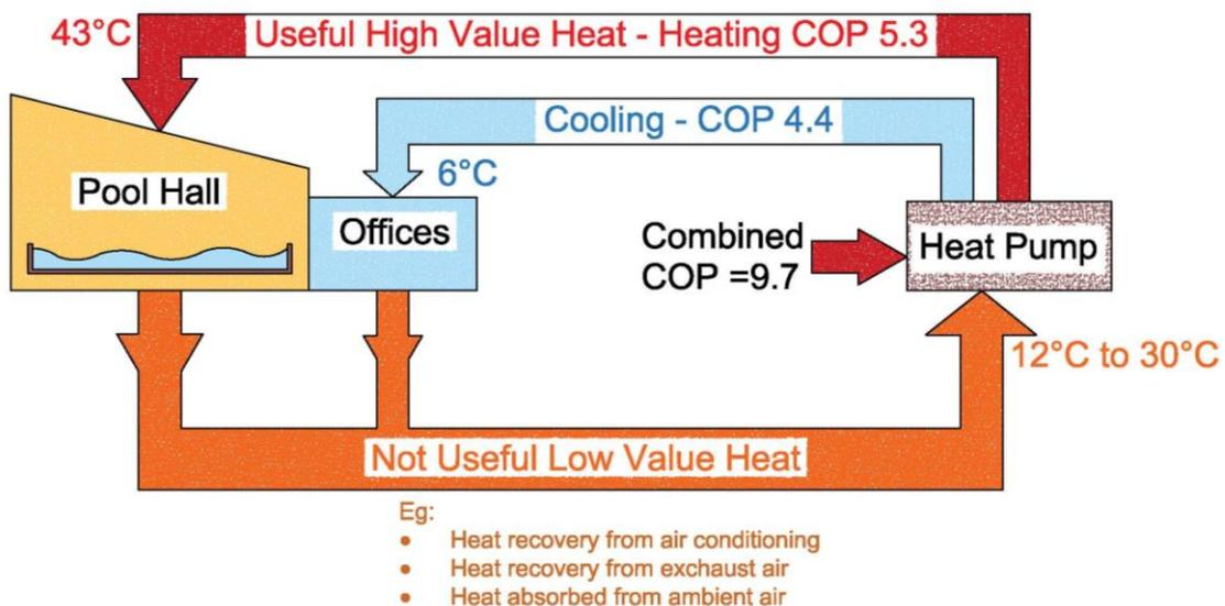
The proposed type of heat pumps use robust industrial components for their compressors, heat exchangers and controls. Because the concept uses water to provide the evaporator input heat and to absorb the condenser discharge heat, these systems have small refrigerant charges which is completely self-contained.
