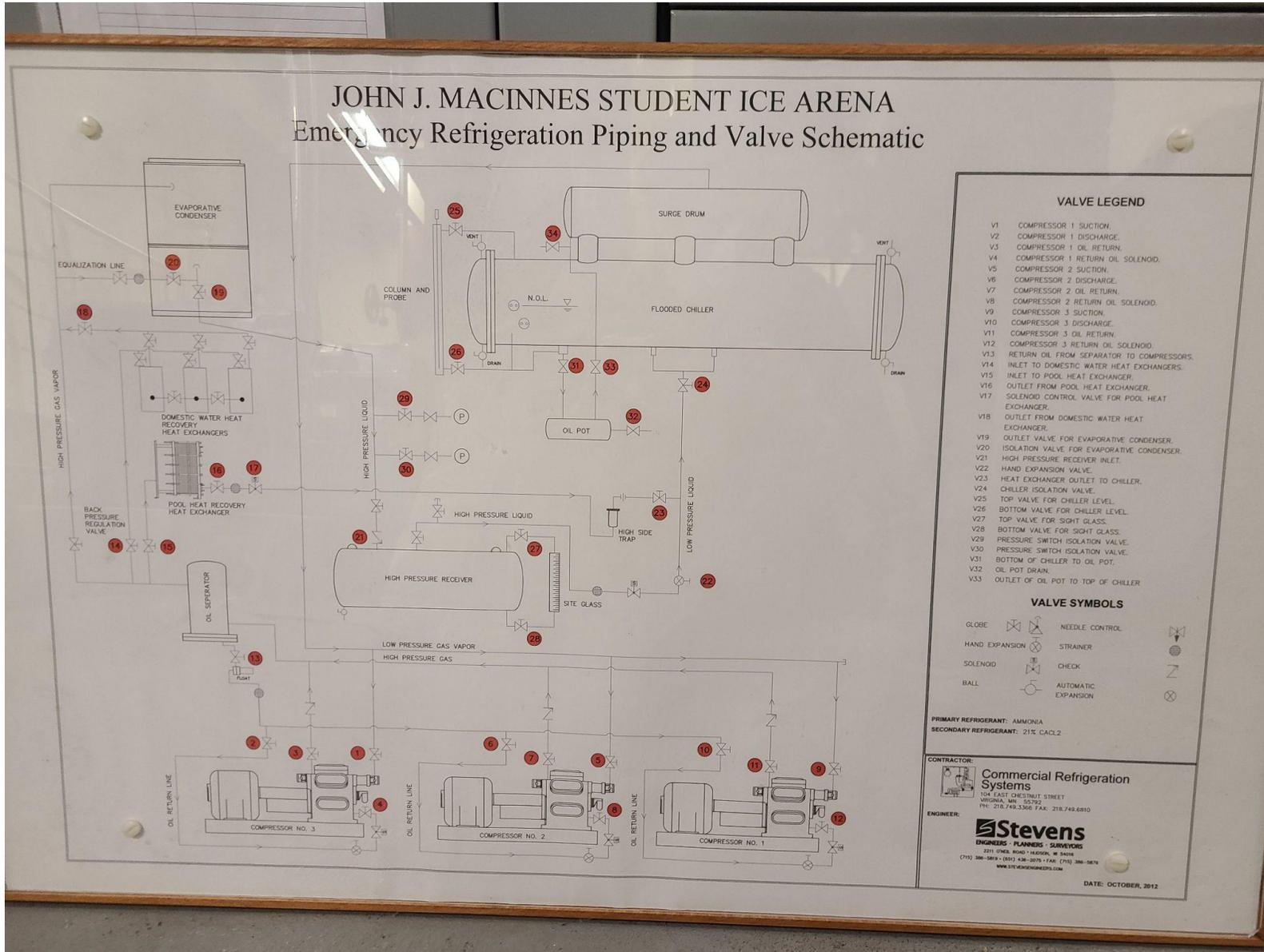
Figure 2 shows the schematic for the entire system. The ice is kept cold with a R-717 refrigerant system, this cools a brine that is pumped through the floor of the ice arena. It has 3 compressors but is designed to only need two even on a 90 degree fahrenheit day, the third is a backup.
